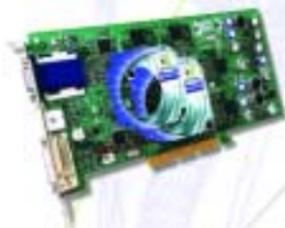
The **NVIDIA Quadro4 750 XGL** offers high-end features at a more aggressive price for outstanding performance. Features include the programmability of the second-generation NVIDIA nfiniteFX™II Engine and 128MB of fast DDR memory.
