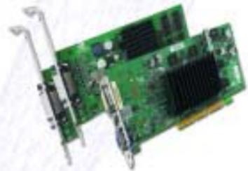
The **NVIDIA Quadro4 380/550/580 XGL** boards provide the fastest entry 3D graphics performance. These low-profile and full-height ATX configurations combine the performance of 64MB of memory and the flexibility of dual-analog, dual-digital, or digital and analog plus TV (380 XGL) displays for maximum on-screen real estate and productivity.
